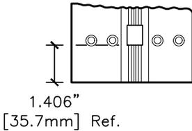
End of hinge to first bearing, both ends.
