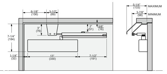
Minimum door rail for mounting closer 7-3/8" (5/8" stop shown) Minimum door rail to bottom of cover 7-3/4" (5/8" stop shown) Backcheck positioning valve in "ON" position
