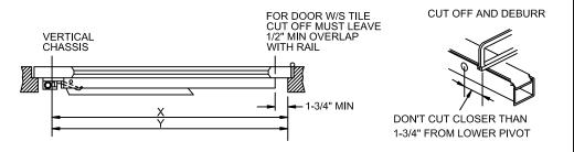
3. DEPRESS ARM INTO RAIL OPENING AND SLIDE RAIL ONTO CHASSIS. LEVEL RAIL AND FASTEN CHASSIS AND MOUNTING PLATE.
