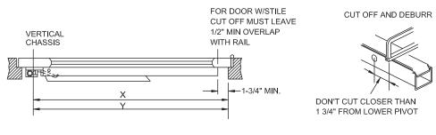
3. DREPRESS ARM INTO RAIL OPENING AND SLIDE RAIL ONTO CHASSIS. LEVEL RAIL AND FASTEN CHASSIS AND MOUNTING PLATE.
