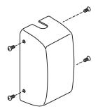
ATTACH COVER TO CHASSIS WITH (4) #8 TRUSS HEAD MACHINE SCREWS.
