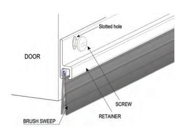
Fastener : Screws Size - #6 x 5/8" PPHSMS
