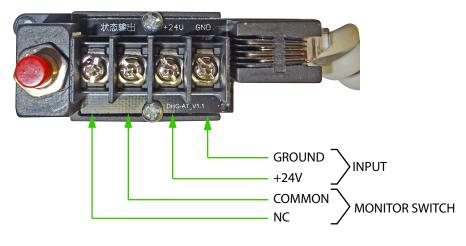
MONITOR SWITCH Switch is Normally Closed when door is in close position Switch is Normally Open when door is in hold open position
