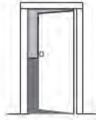
Right Hand Hinges Right Open Inward "RH"
