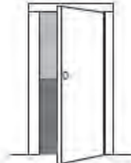
Right Hand Reverse Bevel Hinges Right Open Outward "RHRB"
