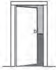
Left Hand Hinges Left Open Inward "LH"
