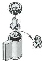
If intending to use a cylinder by a different manufacturer it is advisable to confirm beforehand that the new cylinder is a 6-pin.
