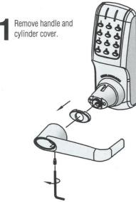
Turn key 90° clockwise and remove cylinder from boss.
