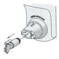
Remove key from cylinder. Hold down the control pin in the end of the cylinder and unscrew the cap.
