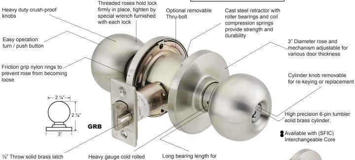
1/2" Throw solid brass latch bolt, reversible and adjustable for flat or beveled doors. UL listed for A Label (3 hour) single swing door Heavy gauge cold rolled spindles add greater strength and security Long bearing length for smooth, wear resistant operation
