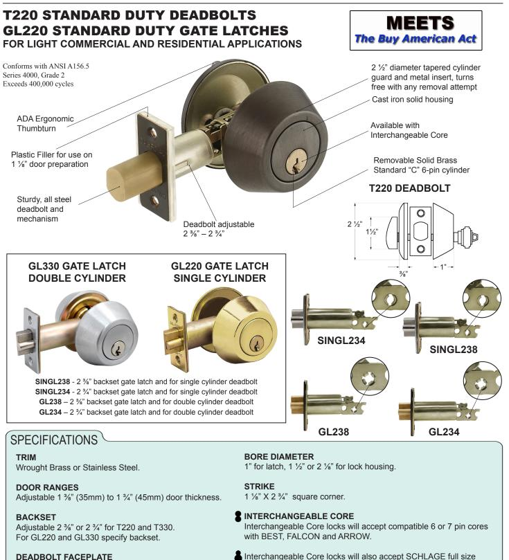
**DEADBOLT FACEPLATE** Latch bolt: Standard 2 ¼" x 1" packed with ½" plastic filler to convert 1" face plate to 1 ½" wide door preparations.
