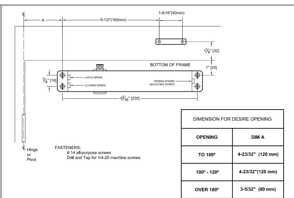
NOTE: ILLUSTRATION SHOWN IS FOR LEFT HAND APPLICATION. FOR RIGHT HAND, REVERSE TEMPLATE. (DOOR CLOSER REGULAR ARM TEMPLATE APPLICATION (PULL SIDE)
