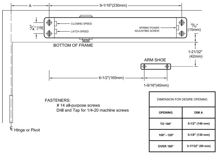
NOTE: ILLUSTRATION SHOWN IS FOR LEFT HAND APPLICATION. FOR RIGHT HAND, REVERSE TEMPLATE. (DOOR CLOSER TOP JAMB TEMPLATE APPLICATION (PUSH SIDE)
