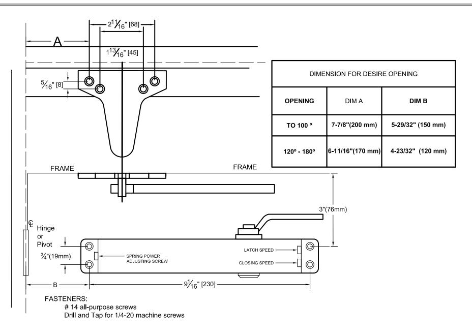
NOTE: ILLUSTRATION SHOWN IS FOR LEFT HAND APPLICATION. FOR RIGHT HAND, REVERSE TEMPLATE. (DOOR CLOSER REGULAR ARM TEMPLATE APPLICATION (PUSH SIDE)
