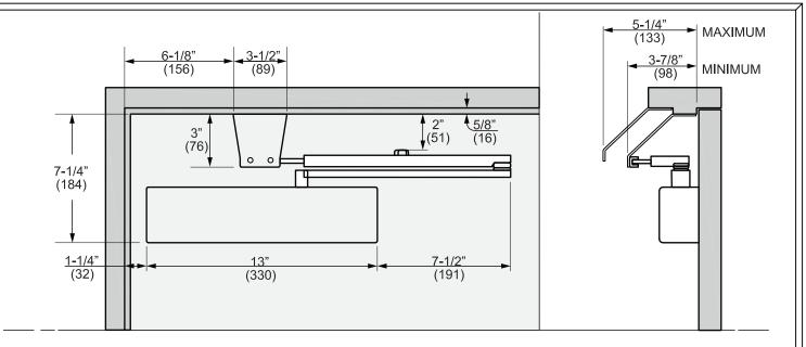
Minimum door rail for mounting closer 7-3/8" (5/8" stop shown) Minimum door rail to bottom of cover 7-3/4" (5/8" stop shown) Backcheck positioning valve in "ON" position
