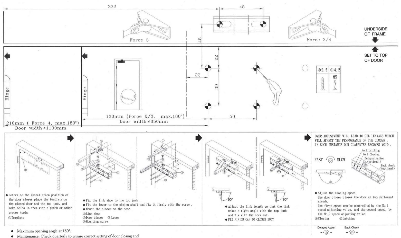
Maintenance: Check quarterly to ensure correct setting of door closing and latching speeds and that fixing screws are tight. A small amount of oil applied to door hinges and the arm joints and rollers will assist performance.
