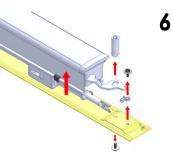
You need to remove two (2) screws, then you can remove the normally open mechanism.
