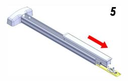
By removing the bump, you can now remove the Push Rall Assembly.
