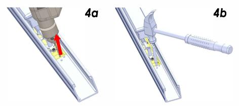
There are two methods to remove the bump. (4a) Electric Drill (4b) Hammer.
