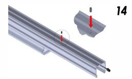
Flip over the Mount Base and push the Kit Assembly to align both kit hole and Mount Base hole, then fasten stop screw.
