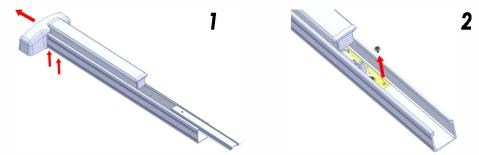
Unfasten fixed screws and remove Device Head.
