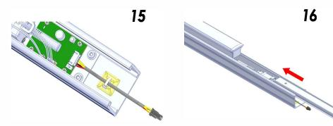
Stick the tie mount and use the cable tie to fix cable in place.
