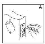
A. Insert latch in hole and keep it parallel to door face. Mark outline and remove latch.
