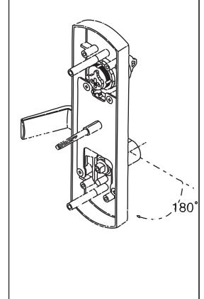
2. Place and fasten cam piece with locked type washer and screw
