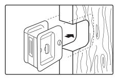
A. Slip lock into notch and position correctly.
