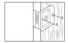
3. A. Tighten machine screws (A) on both side of door.
