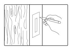
A. Place strike plate on door frame centered over 1" (25mm) hole drilled in step 4D.
