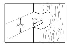
1. A. Mark door with template at desired height. B. Cut out notch.
