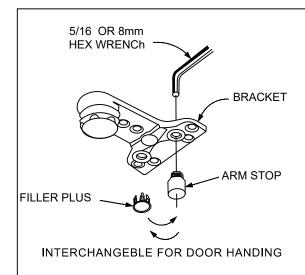
of door (refer to page 1) THE HAND MUST BE CORRECT BEFOR THE BRACKET IS MOUNTED TO THE DOOR STOP (TOP JAMB).
