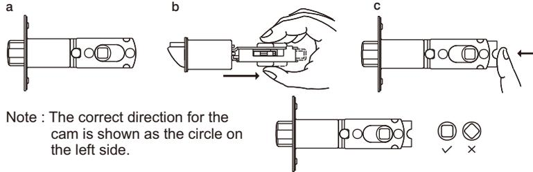
Note : The correct direction for the cam is shown as the circle on the left side.
