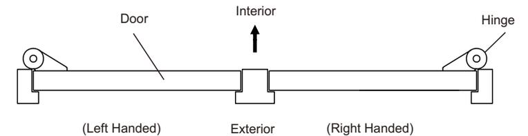
Check that the lever direction meets the door handing. If not, please switch the levers by following steps.
