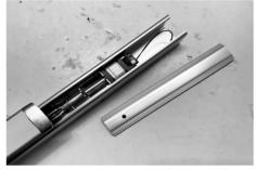
2. Remove the End Cap and shim of the Exit Device.
