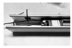
Secure the wire using the cable tie mount for wire management then place the label sticker in an area where its visible.
