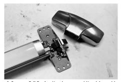
Remove Exit Device Head cover and Head Assembly to access the push bar.
