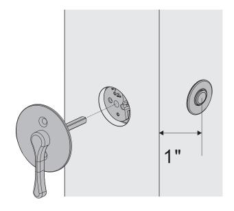
2. Insert trim into spindle hole. Use thumb turn to test lock bolt movement.
