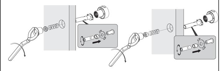
4. Install break-away screw and tighten with Allen wrench. DO NOT OVER TIGHTEN.
