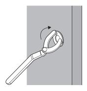
5. Push the button on top and use a screw driver to push through center hole on release to push lock bolt back and unlock the door.
