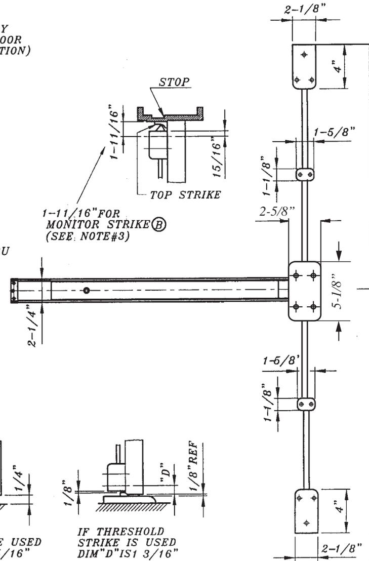
1. SURFACE OF DOOR WHERE EXIT DEVICE IS TO BE APPLIED MUST BE FLUSHED
