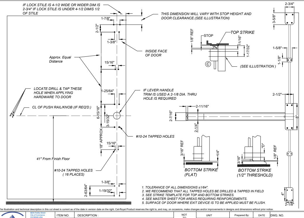
TO Tel.# (323) 888-6601 A L-R O Y A EDT-4130-08/24-1 of 1 **SCALE** FAX # (323) 888-6699 08/12/2024 PRIMARY DIMENSION AF7760V SURFACE VERTICAL ROD FIRE RATED EXIT DEVICE BBT / ADG / CVL WEB SITE SHOWN IN INCHES CAL-ROYAL.COM PAGE 1 OF 1 REV: Ver-01
