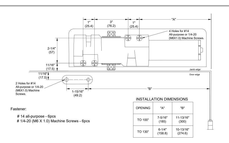
NOTE: Illustration shows RIGHT HAND DOOR configuration. For LEFT HAND DOOR should be installed is symmetry
