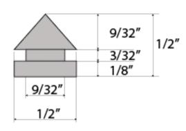
NOTE: Drill 9/32" diameter hole on frame.
